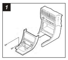
Disconnect the negative battery terminal to prevent an accidental short circuit. Remove (2) screws below the ashtray. Unclip the dash trim bezel. Disconnect the cigarette lighter wiring and remove the bezel. Remove (2) bolts securing the rear of the factory head unit and disconnect the wiring.
