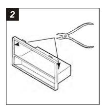
Cut and remove the *SIDE* clips from the *Radio Housing*.
