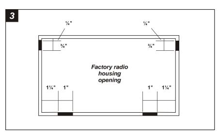
Modify the factory radio housing by trimming the shaded portions of the housing lip. Skip to the Installation Instructions for ALL VEHICLES on Page #11.
