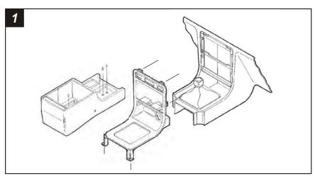
Disconnect the negative battery terminal to prevent an accidental short circuit. Remove the ashtray and (1) ¾" #8 Phillips screw exposed. Open the storage compartment and remove (2) #8 Phillips screws exposed. Remove the cupholder tray and (3) #8 Phillips screws inside. Lift the center console out and remove (2) Phillips screws exposed at the base of the dash trim bezel. Unclip the bezel and remove. Remove (2) hex-head screws securing the factory head unit and disconnect the wiring.
