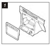
Disconnect the negative battery terminal to prevent an accidental short circuit. Unclip the radio trim bezel and disconnect the clock and climate control wiring. Remove (2) 8mm hex-head screws securing the factory head unit and disconnect the wiring.
