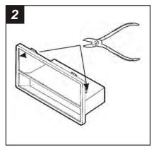
Cut and remove the SIDE clips from the *Radio Housing.*
