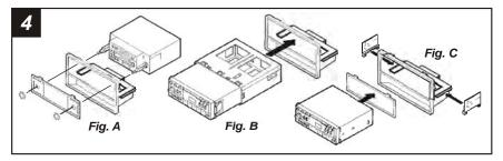
**2-SHAFT HEAD UNITS:** Snap the Faceplate into the **Radio Housing**. Slide the aftermarket head unit into the kit and secure with shaft nuts. (see Fig. A)
