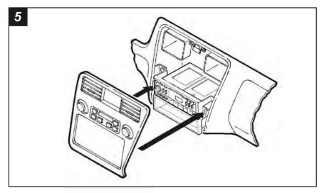
Re-attach the radio trim bezel. (Be sure the clips on the back of the bezel engage the slots on the kit).
