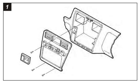
Disconnect the negative battery terminal to prevent an accidental short circuit. Unsnap the clock panel, disconnect the wiring and remove. Remove (1) Phillips screw exposed in the clock cavity. Remove (2) Phillips screws below the factory head unit. Unclip the radio trim bezel and disconnect the wiring. Remove (4) Phillips screws securing the factory head unit assembly and disconnect the wiring. Remove (2) screws securing the factory pocket to the assembly.
