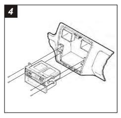
Re-connect the battery terminal and test the unit for proper operation. Mount the head unit/kit assembly to the sub-dash with (4) Phillips screws previously removed.
