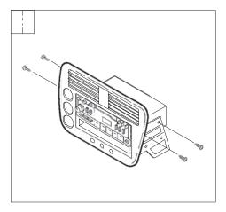
Remove (4) Phillips screws from each side securing the factory head unit to the bracket assembly and remove the unit.
