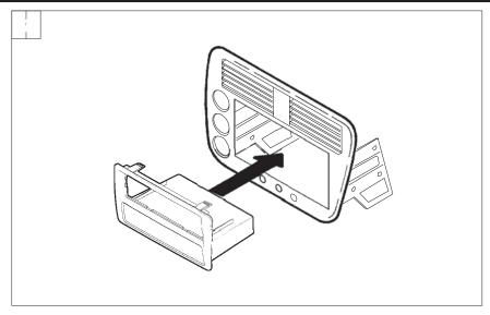
Snap the Radio Housing into the sub-dash.
