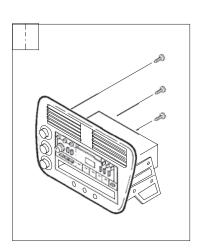
Remove (3) screws securing the climate control pod to the back of the dash trim bezel and remove the pod.
