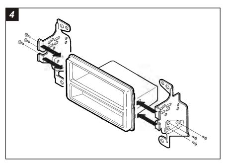
Attach the Mounting Brackets  $\,$  to the sides of the Radio Housing  $\,$  by inserting the slotted Bracket tabs into the slotted Housing tabs. (Be sure the mounting bosses on the Brackets align with the mounting bosses on the Pocket  $\,$ ). Mount the Brackets to the Pocket with (6) #6 x  $\,$ ½"Phillips Flat-Head Screws.
