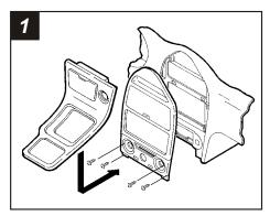
Disconnect the negative battery terminal to prevent an accidental short circuit. Unclip and remove the gear shifter trim bezel and remove (2) Phillips screws exposed below the climate controls. Pull off climate control knobs and remove (2) Phillips screws exposed. Unclip the climate control/factory radio trim bezel and remove. Remove (4) 10mm screws securing the factory head unit and disconnect the wiring.
