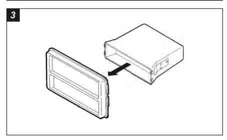
Snap the Pocket onto the back of the Radio Housing.
