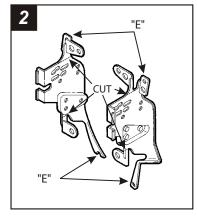
Locate Radio Housing "E". Using the dotted lines as a guide, cut and remove all tabs on the Mounting Brackets EXCEPT tabs "E". Skip to the Installation Instructions for ALL VEHICLES on Page #2.
