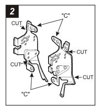
Locate Radio Housing "C". Using the dotted lines as a guide, cut and remove all tabs on the Mounting Brackets EXCEPT tabs "C". Skip to the Installation Instructions for ALL VEHICLES on Page #2.
