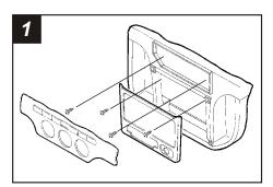
Disconnect the negative battery terminal to prevent an accidental short circuit. Remove the climate control knobs and (2) Phillips screws exposed. Unclip and remove the climate control trim bezel. Depress the side clips securing the climate control panel and move the panel to access (2) Phillips screws from the top of the factory radio brackets. Remove the ashtray. Unclip and remove the radio trim bezel. Remove (2) Phillips screws from the bottom of the radio brackets and disconnect the wiring.
