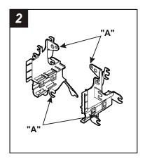
Cut and remove all tabs on the Mounting Brackets EXCEPT tabs "A". (The tabs can be identified by the stamped letter by each tab). Skip to the Installation Instructions for ALL VEHICLES on Page #3.
