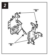
Cut and remove all tabs on the Mounting Brackets EXCEPT tabs "B". (The tabs can be identified by the stamped letter by each tab). Skip to the Installation Instructions for ALL VEHICLES on Page #3.
