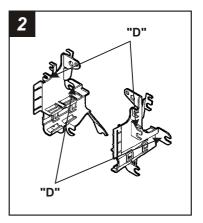
Cut and remove all tabs on the Mounting Brackets EXCEPT tabs "D". (The tabs can be identified by the stamped letter by each tab). Skip to the Installation Instructions for ALL VEHICLES on Page #3.
