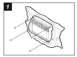
Disconnect the negative battery terminal to prevent an accidental short circuit. Remove (4) 3/16" Allen Screws from the radio trim bezel and remove the bezel. Remove (4) 10mm bolts securing the factory head unit and disconnect the wiring.
