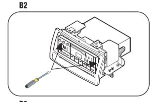
Re-connect the battery terminal and test the unit for proper operation. Snap the factory head unit trim bezel over the kit by engaging the (4) bracket tabs ("A") and (3) Housing bosses ("B") to the back of the bezel. Slide the assembly into the subdash and mount with (4) 10 mm bolts previously removed in step #1. Re-assemble the dash. (See Fig. B3)
