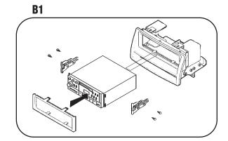
**NOTE:** To remove the mounted head unit, unclip and remove the ISO Trimplate. Using a small flat-blade screwdriver, disengage the side clips securing the ISO Brackets to the Radio Housing. (See Fig. B2)
