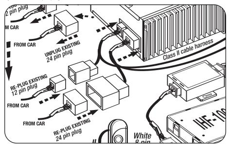
4) Insert the 12 pin plug on the Class 2 cable into the rear of the radio.
