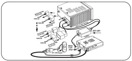
**10)** Install the IHF-1000 microphone in an appropriate location (see IHF-1000 instructions), route the wire to the IHF-1000 harness, and attach the microphone connector to the harness.
