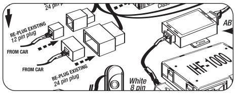
**6)** Connect the 12 pin cap on the Class 2 cable to the 12 pin plug connected to the vehicle (the connector that was removed from the back of the radio).
