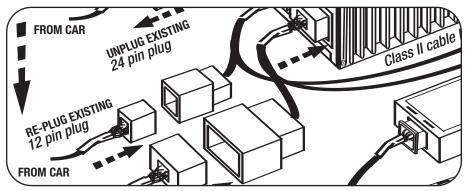
7) Connect the white 10-pin plug on the Class 2 cable to the ABTI-GM1 module.
