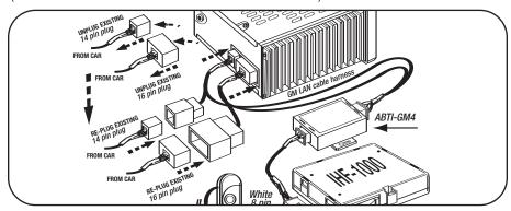
7) Connect the white 10-pin plug on the ABTI-GM4 cable to the ABTI-GM4 module.
