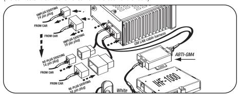
**6)** Connect the 16 pin cap on the ABTI-GM4 cable to the 16 pin plug connected to the vehicle (the connector that was removed from the back of the radio).
