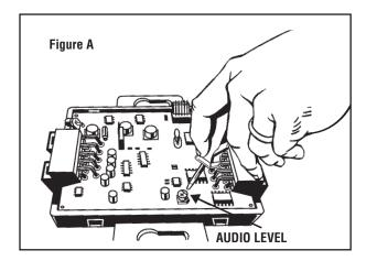
When using the CHTO-03 with a radio that has a high audio pre-out voltage, usually greater than 2 volts, the audio signal may become distorted. To resolve this follow these steps:
