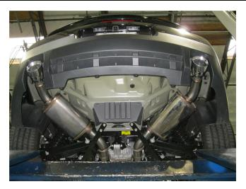
**Step 4.** Next attach the driver and passenger side Muffler Assemblies to the Mid Pipe Assemblies using the supplied 3.00" clamps and by fitting the hangers into the rubber insulators. Complete the installation by re-installing all the braces that were removed.
