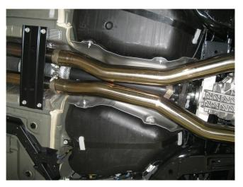
**Step 3.** Next attach the Mid Pipe Assemblies to the X-Pipe using the supplied 3.00" clamps. Loosely connect the Mid Pipes using the supplied 3/8 fasteners at the brackets. The D/S bracket should be on top of the P/S bracket per the photo. .
