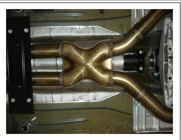
**Step 2.** Begin installation of the new system by loosely attaching the X-Pipe Assembly to the catalytic converter outlets using the OEM clamps.
