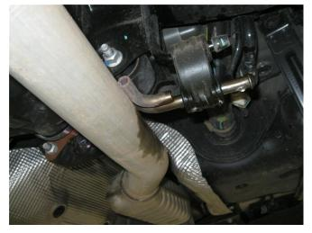
**Step 2.** Disengage rubber insulators (Do not damage insulators as they will be used in the new installation) and remove system from the vehicle.
