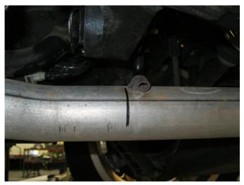
**Step 1.** Removal of this exhaust system requires cutting and de-burring the pipe directly in front of the hanger behind the catalytic converter. (cut at line location)
