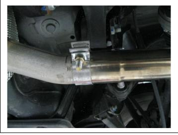
**Step 3.** Begin installation of your new MAGNAFLOW system by attaching the Inlet Pipe Assembly to the cut outlet behind the catalytic converter using the supplied 2.25" clamp (Keep all clamps loose until final adjustment) and insert hanger into rubber insulator.
