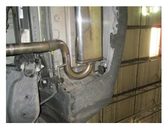
**Step 4.** Next, install the Muffler Assy to the Inlet Pipe Assembly using a supplied 2.25" clamp and fitting the hangers into the rubber insulators.
