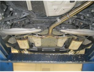
**Step 3.** Next Install the Extension Pipe Assembly to the outlet of the Resonator Assembly using the supplied 2.50" clamp. Then install the Y-Pipe Assembly to the Extension Pipe Assembly in the similar fashion using the supplied 2.50" clamp, and fitting the welded hangers into the rubber insulators.
