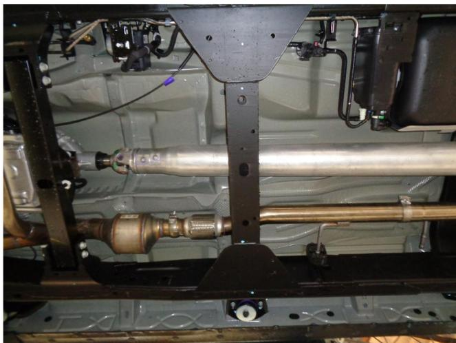
**Step 2.** Begin installation by loosely attaching the Inlet Pipe Assembly to the catalytic converter ball flare using the OEM hardware. Engage the welded hanger to the rubber insulator.
