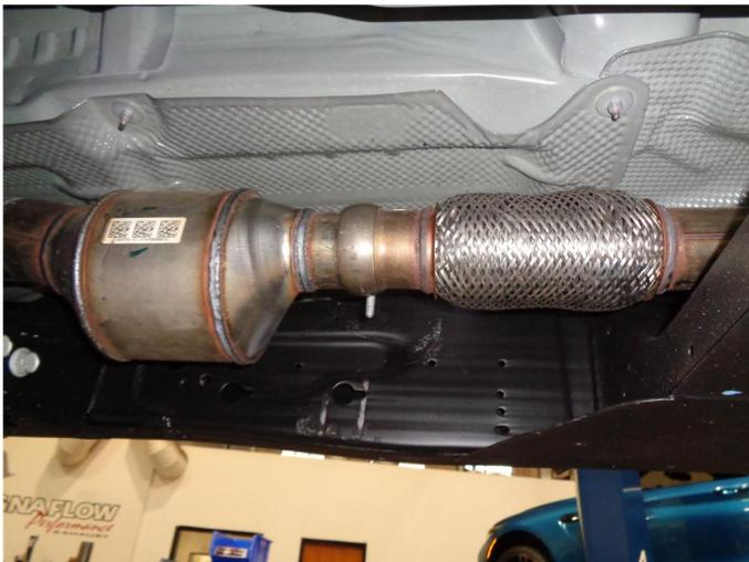
**Step 1.** To remove the OEM exhaust loosen the clamp at the ball flare junction attaching the inlet pipe to the catalytic converter outlet. Working front to rear disengage all welded hangers from the rubber insulators. Be sure to retain all mounting hardware as it will be needed to install your new MAGNAFLOW system.
