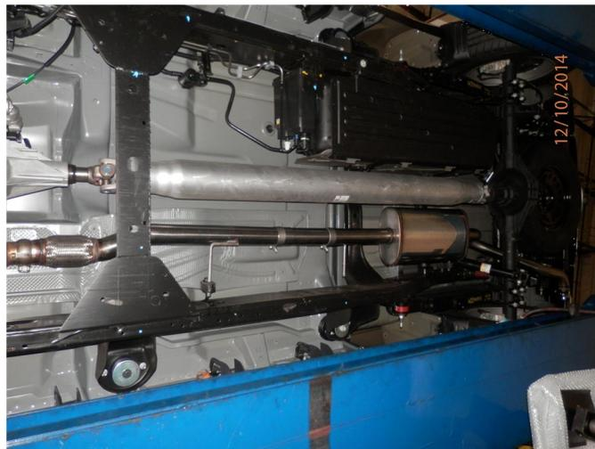
**Step 3.** Only Crew Cab with 78.8in. Bed vehicles will require the 12.5" Extension Pipe to be fitted between the Inlet Pipe Assembly and the Muffler Assembly. Loosely attach the Muffler Assembly using the supplied clamps. Engage all welded hangers to the rubber insulators.
