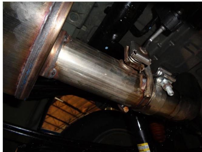
**Step 4.** Next loosely attach the Tail Pipe Assembly to the valve outlet on the Muffler Assembly using the supplied clamp. Engage the welded hanger to the rubber insulator.
