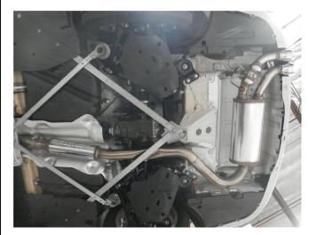
**Step 5.** Loosely attach the Muffler Assembly to the Inlet Assembly using the supplied clamp. Engage all welded hangers to the rubber insulators.
