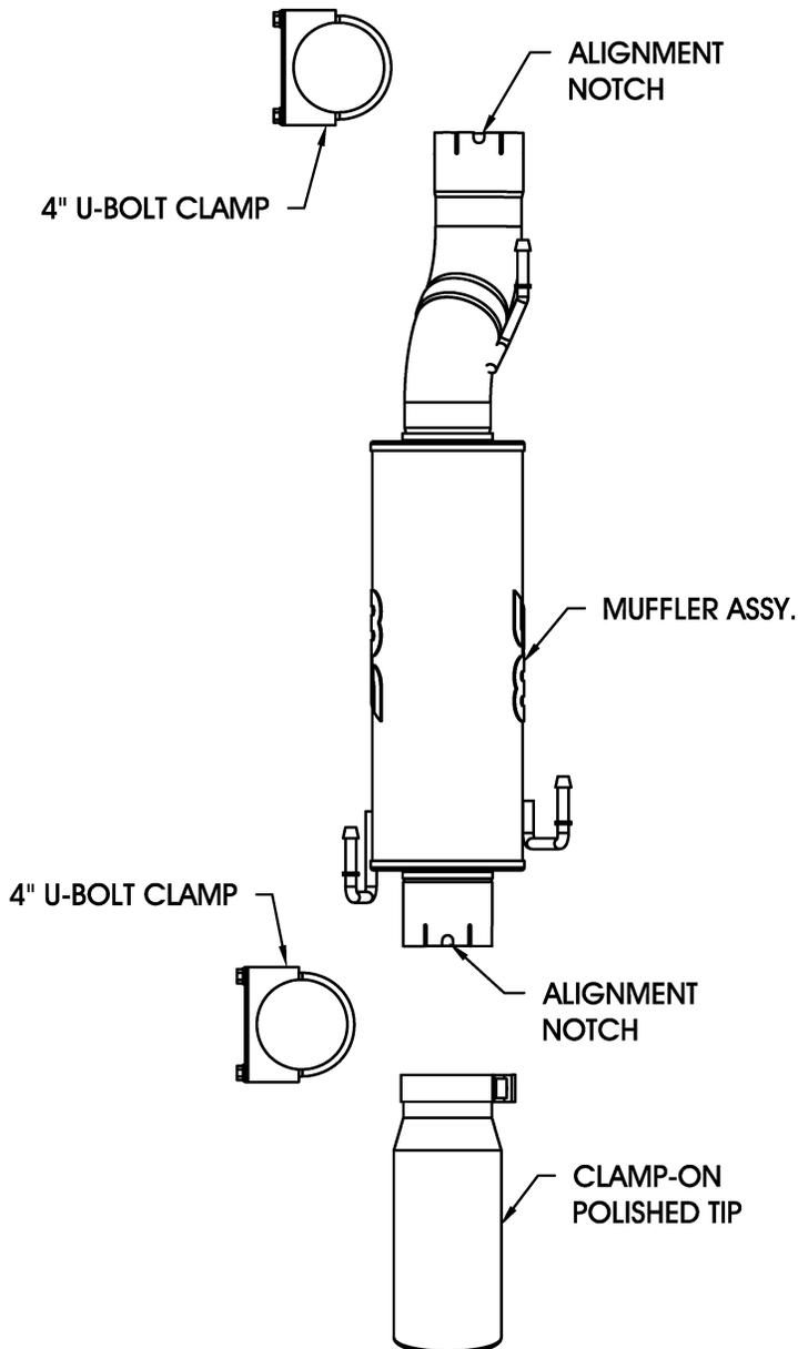
**Step 1:** (Carefully read all instructions before installation) Disconnect the vehicle's battery before removal of the OEM exhaust system. This will allow the computer to reset itself with the new system, and prevent electrical accidents. Remove the OEM muffler by unbolting the U-bolt clamps and disengaging the muffler from the OEM rubber insulators. Be careful not to damage the OEM rubber insulators, as they will be re-used to mount the new system.
