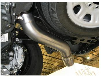
**Step 3.** Next Install the Tail Pipe Assembly in a similar fashion using the supplied 5.00" clamps and by fitting the welded hangers into the rubber insulators.
