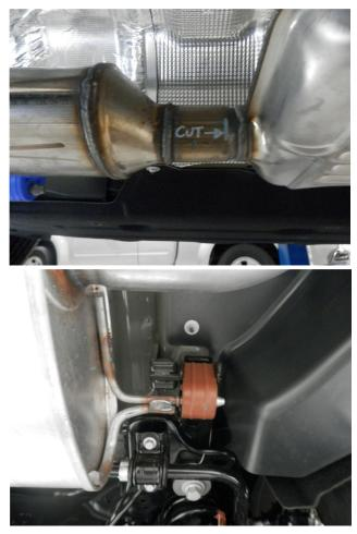
**Step 1.** To remove the OEM exhaust begin by cutting the tubing approximately 2.00" behind the weld on the catalytic converter. Once cut, working front to rear, disengage the hangers from the rubber insulators and remove the system. Do not damage or discard the rubber insulators as they will be re-used to install the new Magnaflow system.
