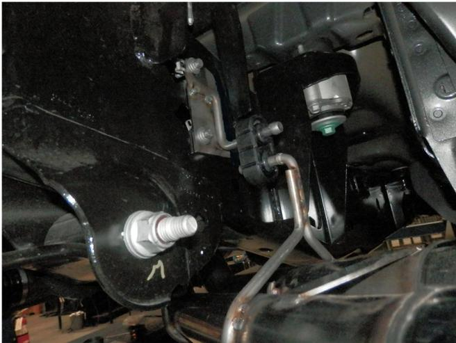
**Step 5.** Locate the two square holes in the passengers side of the vehicles subframe. Attach the two supplied U-type panel nuts as shown in the diagram. Loosely bolt the supplied Hanger Bracket Assembly to the panel nuts using the supplied bolts.
