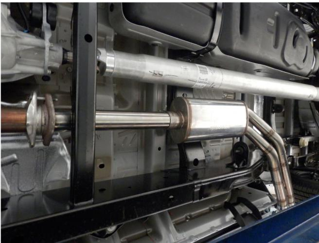
**Step 6.** Install the Muffler Assembly and loosely secure using the supplied 3.00" clamp. Attach the Hanger Bracket Assembly to the welded hanger using the supplied rubber insulator.
