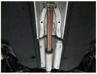
**Step 2.** Begin installation of the new system by fastening the Resonator Assembly inlet to the catalytic converter using the OEM fasteners and fitting the hanger into the rubber insulator (Leave all clamps and fasteners loose for final adjustment of the complete system.)
