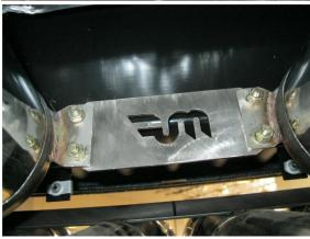
**Step 3.** Next, Loosely attach the Muffler Assemblies to the Inlet pipes using the provided 3.00" clamps. You will then need to fasten the provided cross bracket in place between the two muffler assembles using the provided 1/4" fasteners. Insert all hangers into the rubber isolators. At this point you can re-install the rear valance.
