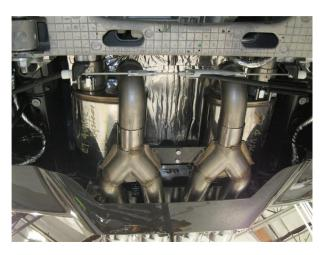
**Step 4.** Once the rear valance is back in place, loosely fasten the Tip sub-assemblies together while on the ground using the supplied fasteners. Now you can attached the Tip assembly to the Muffler assemblies using the provided 2.50" clamps. Plug the wiring into the valve motors checking for cleareance.
