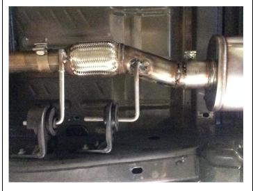
**Step 2.** Before installing your new MAGNAFLOW system the OEM spare tire and spare tire heat shield must be permanently removed. Install the new system by attaching the Inlet Pipe Assembly to the OEM catalytic converter outlet pipes using the existing clamp and hardware. Locate the welded hanger to the rubber insulator. Leave all clamps and fasteners loose for final adjustment of the complete system once installed.
