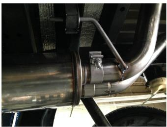
**Step 4.** Install both the Over Axle Pipes using the supplied 2.50" clamps. Locate the welded hanger to the OEM rubber insulator.
