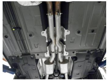
**Step 5.** With both valve assemblies cut from the OEM system, loosen the band clamps attaching the mufflers to the OEM tips. Both tailpipe sections may now be removed. Loosen the two OEM clamps at the outlet of the catalytic converters then carefully remove the rest of the exaust system. Disengage all welded hangers from the rubber insulators. Do not discard or damage the clamps or rubber insulators as they will be needed to install the new system.
