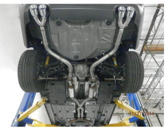
Step 9. To install the Quad Tip option supplied you will first need to remove the OEM tips from the vehicles valence. Remove the four bolts attaching each tip. Once the tips are removed install the Quad Tip Tailpipe Assemblies using the supplied 3.00" clamps. Locate both welded hangers to the rubber insulators.
