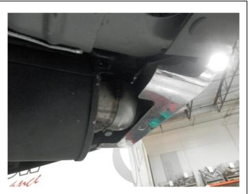
Step 8. To retain the OEM tips on your vehicle select the two OEM Tip Assemblies. The drivers side will be slightly longer. Loosely attach each pipe inlet to the Over Axle Pipes outlets using the OEM clamps. Engage the welded hangers for each to the rubber insulators.
