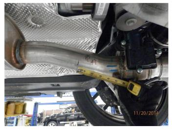
**Step 4.** For the passengers side cut 4.50" in front of the welded hanger forward of exhaust control valve as shown in the attached picture.
