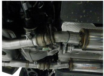
Step 7. Next, loosley fasten the X-Pipe Muffler Assembly outlet pipes to the OEM control valve outlet that you have just cut using the supplied 2.75" clamps. Attach the two Inlet Pipes in a similar fashion to the outlet of the control valve. At this point you have two options for tips. Magnaflow supplies a quad tip setup or an extension pipe assembly to allow for the original OEM tips. Select the desired option before continuing the installation.
