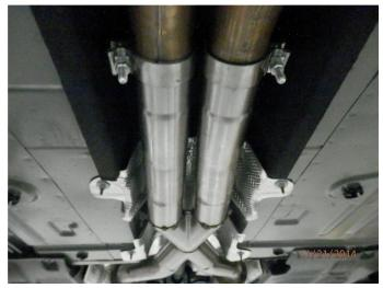
**Step 6.** Begin installation of the new system by slipping the inlet pipes of the X-Pipe Muffler Assembly over the catalytic converter outlets. Loosely secure using two of the suppled 2.75" clamps. Orientation of the Muffler Assembly can be confirmed by the MF logo being "upright" after installation.
