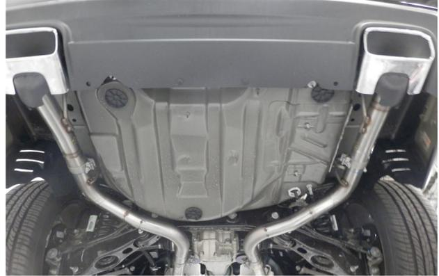
**Step 3.** Attach the Mid-pipes to the Resonator Assembly with supplied 2.50 Clamps and fit hangers into rubber insulators. Remember to re-attach the ground strap to the hanger. At this point you have two options for tips. Magnaflow supplies a straight tip setup that can be run into the existing valance surround and held in place with hangers and the installation is complete.
