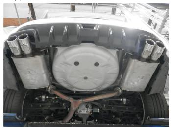
**Step 2.** Unbolt both flange junctions attaching the muffler assemlies. Next working front to rear extract the hangers from the rubber insulators and remove the OEM system. Retain insulators and clamps as they will be used to install the new system.
