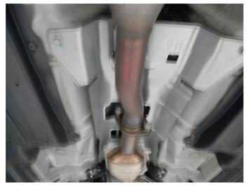
**Step 1.** Begin removing the OEM exhaust system by unbolting the flange on the outlet of the catalytic converter to the inlet pipe.
