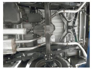
**Step 2.** Begin installing of the new system by attaching the Inlet Pipe Assembly to the outlets of the OEM system using the OEM hardware. Next attach the Mufler Assembly to the inlet pipes with supplied clamps and insert the hangers into the rubber insulators. Keep all clamps loose for final adustment of the system.
