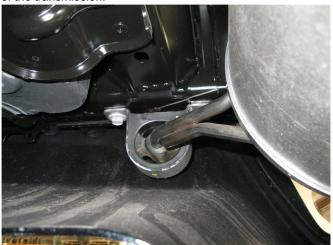
**Step 5.** Unbolt both hanger brackets located either side of the muffler assemblies. Unclip the plugs connecting the valve motor assemblies. Disconnect the wiring harness on both sides of the tail pipe assemblies.
