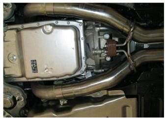
**Step 4.** On vehicles with automatic transmission you will need to disconnect the shift linkage located on the drivers side of the transmission.
