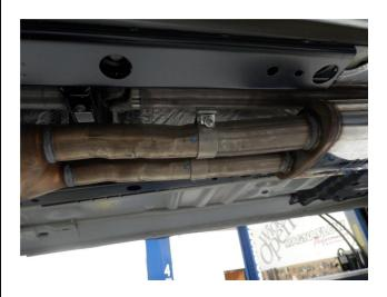
**Step 2.** To install the new Magnaflow exhaust system begin by attaching the Resonator Assembly to the cut and de-burred outlet of the OEM system using the supplied 2.25" clamps. Leave all clamps loose until final adjustment of the system.
