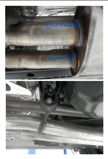
**Step 1.** To remove the OEM exhaust begin by cutting the tubing at the weld junctions in front of the OEM resonator. Once cut, working front to rear, disengage the hangers from the rubber insulators and remove the system. Do not damage or discard the rubber insulators as they will be re-used to install the new Magnaflow system.
