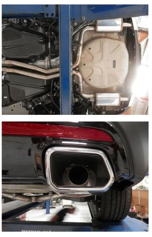
**Step 4.** Complete the installation by attaching the Muffler Assemblies to the Mid-Pipes using a 2.50" clamps and fitting the tailpipes into the openings in the rear valance and the hangers into the rubber insulators.
