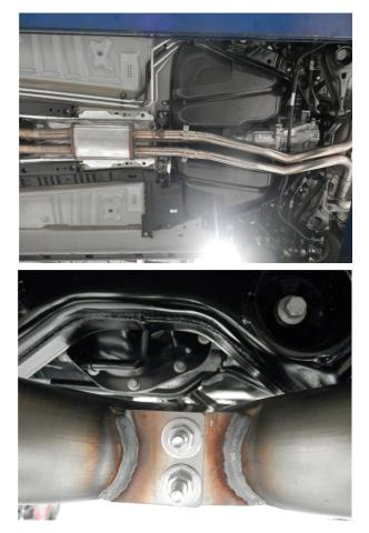
**Step 3.** Next attach the Mid-Pipe Assemblies to the Resonator Assembly using the supplied 2.50" clamps. At this time also use the supplied 5/16" fasteners to connect the Mid Pipe Assemblies.
