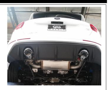
**Step 7.** Once a final position has been chosen for the new exhaust system, evenly tighten all clamps from front to rear using the torque specifications on page one of the instructions. Inspect all fasteners after 25-50 miles of operation and re-tighten if necessary.
