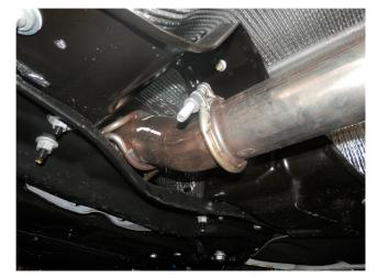
**Step 2.** To remove the OEM exhaust system begin by loosening the clamp located behind the front crossmember. Working from front to rear disengage all welded hangers from the rubber insulators. Retain all mounting hardware as it will be needed to mount your new MAGNAFLOW system.
