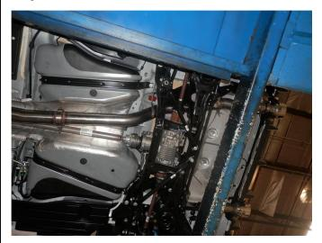
**Step 5.** Next attach the Mid Pipe assembly to the Inlet Pipe using the supplied 3.00" V-clamp and engage the hanger into the rubber insulator.
