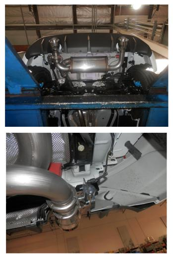
**Step 6.** Loosely install the Muffler Assembly using the supplied clamp. Attach the welded hangers to the rubber insulators. Re-attach the electrical connector to the exhaust valve motor.
