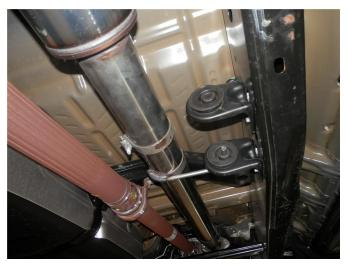
**Step 4.** Loosely install the supplied Hanger Clamp Assembly to either the Inlet Pipe Assembly or the Extension Pipe, depending on your vehicle configuration. Locate the welded hanger to the secondary rubber insulator as shown.
