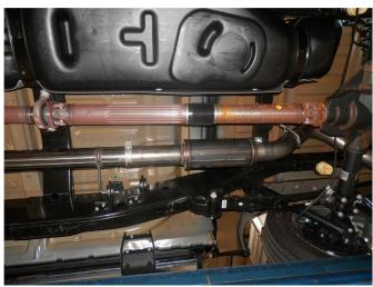
**Step 5.** Next loosely install the Muffler Assembly to the Inlet Pipe Assembly or Extension Pipe using the supplied clamp. Engage the welded hanger to the rubber insulator.
