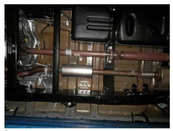
**Step 1.** To remove the OEM exhaust loosen the factory clamp in front of the muffler, loosen the bolts attaching the inlet pipe assembly to the inlet flange junction. Rotate the extension pipe to release the muffler inlet locking boss. Remove the inlet flange bolts. Working front to rear disengage all welded hangers from the rubber insulators. Be sure to retain all mounting hardware as it will be needed to install your new MAGNAFLOW system.
