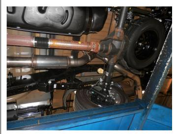
**Step 6.** Loosely install the Tail Pipe Assembly using the supplied clamp. Engage the welded hanger to the rubber insulator.
