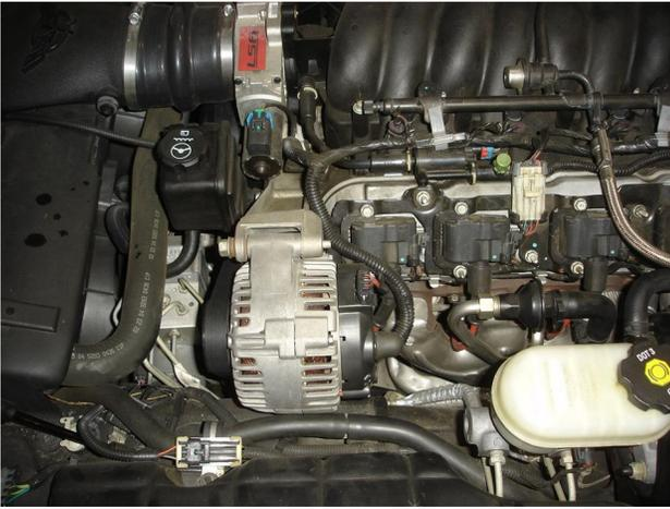
**Step 7.** Using a 15mm socket unbolt the alternator and remove. After alternator has been removed repeat passenger side process to remove the coil pack bracket.
