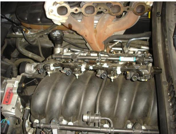
**Step 9.** Using a 13mm socket unbolt both manifold and remove. While removing both manifolds disconnect the O2 sensor plug. Unbolt and remove the O2 sensor cable from the OEM manifold using a 7/8" wrench and bolt it onto your new header assemblies.
