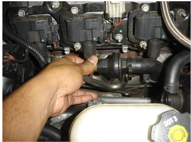
**Step 5.** Disconnect the hose from the EGR pipe on the driver side and remove.
