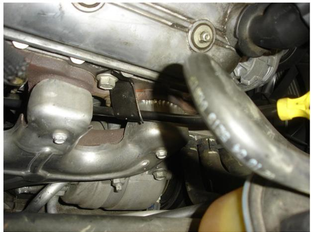
**Step 4.** Using a 15mm socket remove the dipstick assembly.
