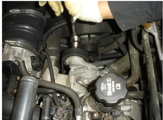
**Step 6.** Release the pressure on the drive belt tensioner with a 15mm socket and remove the serpentine belt.
