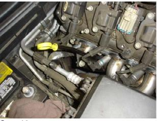
**Step 10.** On the passenger side with your new header installed, you will notice a bracket located on one of the tubes. You will need to reinstall the dipstick assembly to that bracket using the OEM bolt and nut provided with a 17mm socket. Reinstall both coil pack brackets and sparkplug wires to the coil pack and plugs. Reconnect both O2 sensors. Next reinstall the alternator and serpentine belt. Then reconnect the motor covers.
