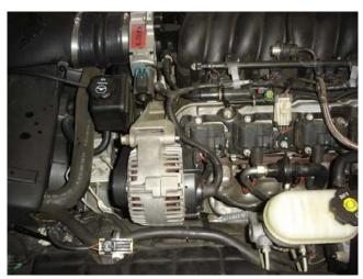
**Step 5.** Using a 15mm socket unbolt the alternator and remove. After alternator has been removed repeat passenger side process to remove the coil pack bracket.
