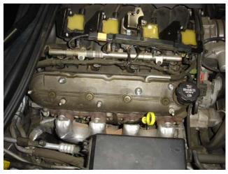
**Step 3.** Remove all spark plug wires from the coils and the plugs, and then set aside. On the passenger side unbolt the coil pack bracket using a 10mm socket and gently flip the assembly towards the upper part of the motor.
