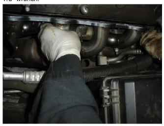
**Step 9.** Reinstall the O2 sensors on your new header assemblies. With the supplied gaskets and header bolts install your header assemblies with a 10mm socket to the manufacturers torque specifications.
