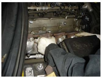
**Step 8.** Unbolt and remove both driver and passenger side manifolds with a 10mm socket. Remove the O2 sensor from the manifolds using a 7/8" wrench.
