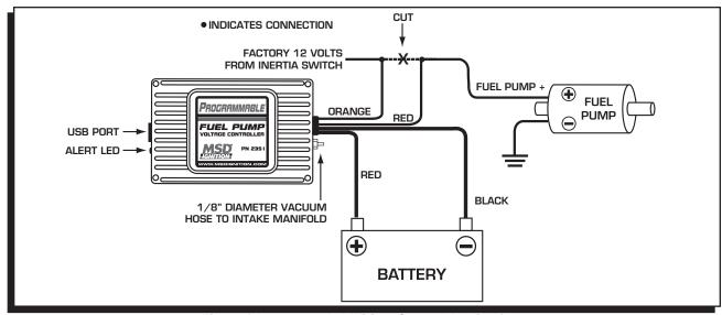
Figure 1 Recommended Wiring, General Application.
