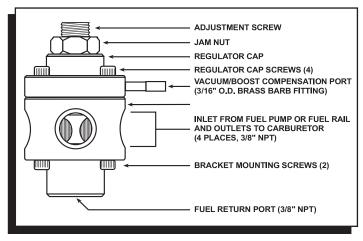
This regulator is equipped with a vacuum/boost compensation port (brass barb fitting) that can be used to momentarily decrease fuel pressure (vacuum compensation) at idle and part throttle, or increase fuel pressure under blower boost (boost compensation). While it is not necessary to connect a hose to the vacuum/boost compensation port, it may be beneficial in some cases. However, the small plug on the barb must be removed before use.
