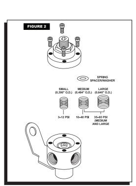
The regulator may be mounted at any angle. For maximum efficiency, mount the regulator as close as possible to the carburetors or fuel injection systems. **DO NOT mount the regulator on or near exhaust manifolds.** A bracket is provided for convenient mounting under an intake bolt.
