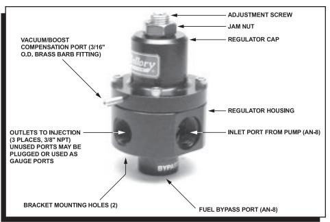
(vacuum compensation) at idle and part throttle, or increase fuel pressure under blower boost (boost compensa- tion). While it is not necessary to connect a hose to the vacuum/boost compensation port, it may be beneficial in some cases. However, the small plug
