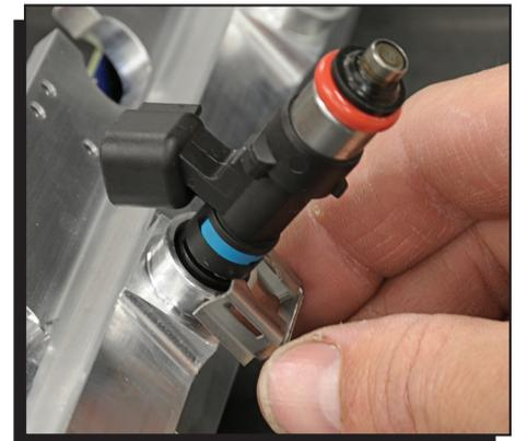
**Figure 6 Installing the Injectors.**
