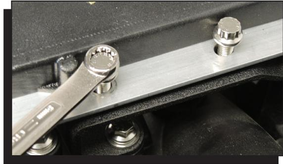
Figure 8 Tighten the Fuel Rail Bolts.
