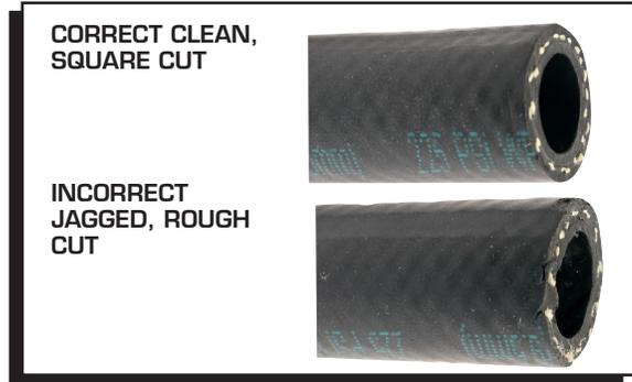
**Figure 11 Severing the Hose Properly.**
