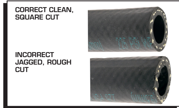
Figure 24 Severing the Hose Properly.
