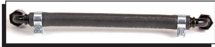
Figure 23 Installing Fuel Hose to AN Fittings.
