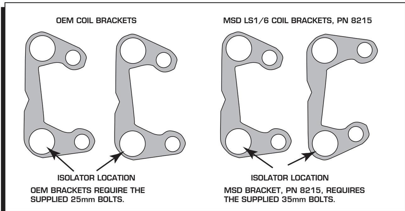
Figure 3 Installing the Isolators.
