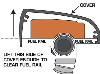
2. When the cover is clear of the fuel rail push the cover towards the manifold until it disengages from the lip of the rail
