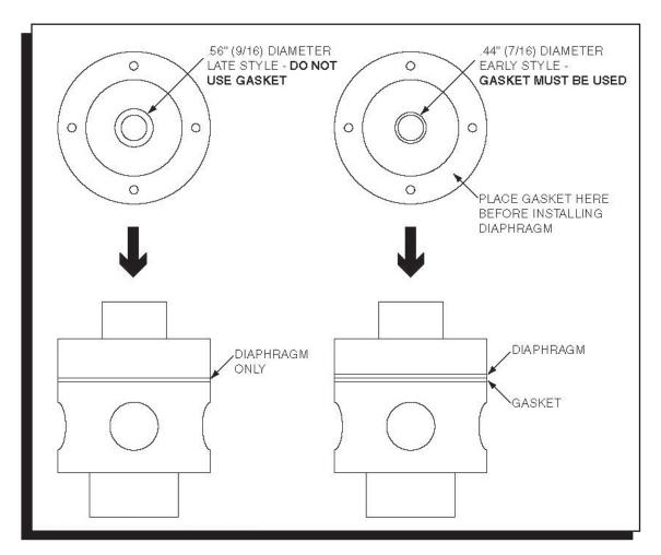
**TECH NOTE:** This gasket does not require the use of silicone.
