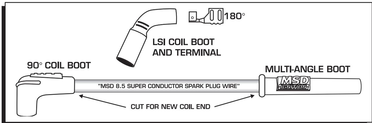
Figure 1 Choosing the Spark Plug Boots and Terminals.
