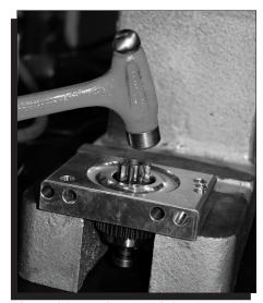
Figure 1 Removing the Pinion Assembly.
