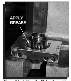
Figure 2 Installing the Pinion Assembly.
