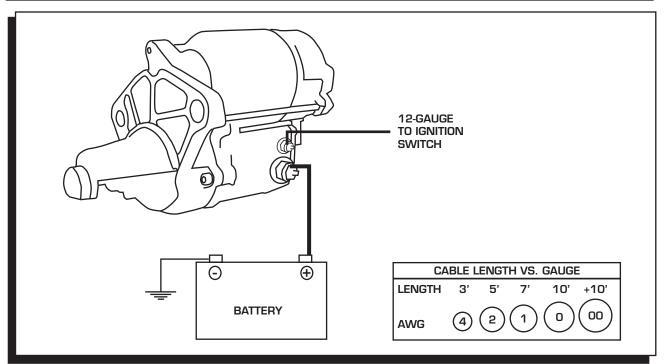
Figure 1 Wiring the Starter.
