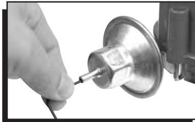
Figure 2 Adjusting the Vacuum Advance.
