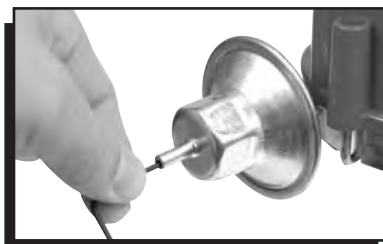
Figure 2 Adjusting the Vacuum Advance.
