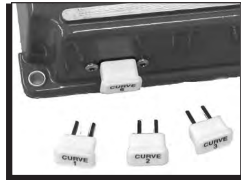
Figure 3 Timing Curve Modules.
