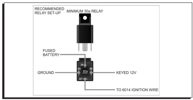
**Figure 3 Recommended Relay Set-Up**
