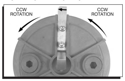
The reason for this modification is because voltage will travel to and from the sharpest point of the rotor tip. By rounding the leading edge of the Tip, the voltage will jump from the sharp point (trailing edge) of the tip which will be closer to the spark plug wire terminal when the timing is retarded. This will produce proper spark distribution even when the timing is retarded (which alters the rotor phasing).
