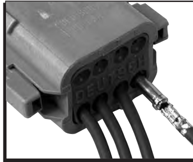
Figure 3 Installing the Terminal.
