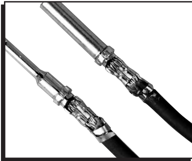
Figure 2 Terminals Crimped to the Wires.
