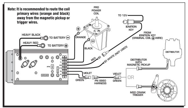
Figure 3 Wiring the Pro Power Coil.
