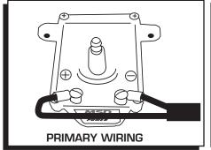
Figure 1 Correct Routing.
