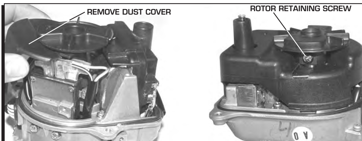
Figure 4 Replacing the Rotor.
