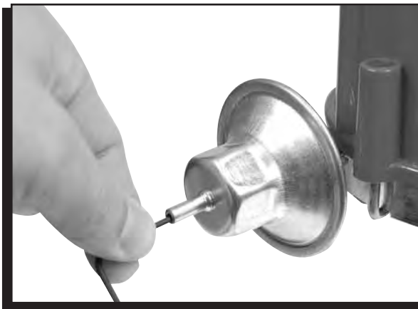
Figure 3 Adjusting the Vacuum Advance.
